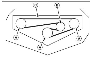
Figure 51. Spindle Drive Belt Removal
